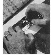
OLD METHOD of numbering electrical circuit boards at Livermore Laboratory was done manually using this special lettering pen. Information was copied directly from engineering drawings and took up to two and a half days to complete. short circuit."
